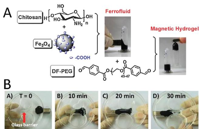
**Fig. 6.** (A) The preparation of the magnetic CP hydrogel. (B) The magnetic hydrogel passing a channel driven by a magnet. Reprinted with permission from ref. [41]. Copyright 2012, Royal Society of Chemistry.
