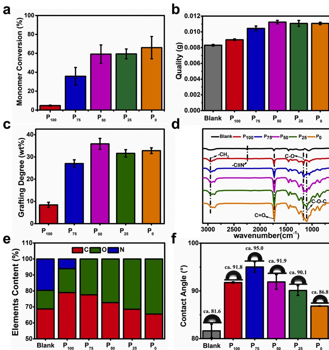
**Fig. 1.** The net mass change and structure characterization of surface photografting with different coating rates. (a) Monomer conversion, (b) net mass, (c) grafting degree, (d) ATR-FTIR Spectrum (e) EDS, and (f) water contact angle.
