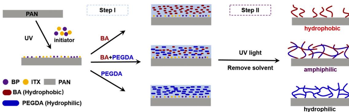
**Scheme 1.** Process of surface photografting. UV light was used to initiate polymerization and grafting of BA and PEGDA monomers onto PAN surface in two steps.
