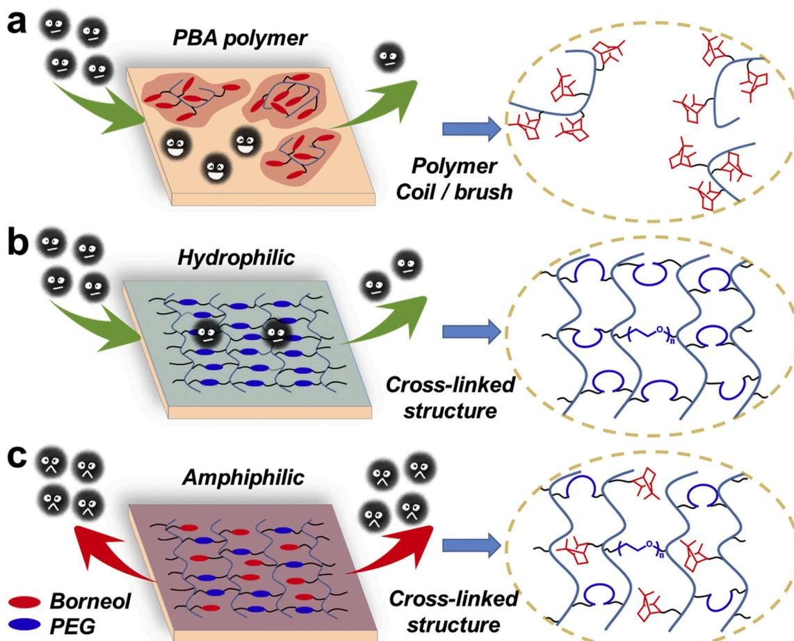
Scheme 2. Schematic representation of the fungal repelling mechanism of P<sub>100</sub> (a) P<sub>0</sub> (b) and P<sub>50</sub> (c) coatings.
