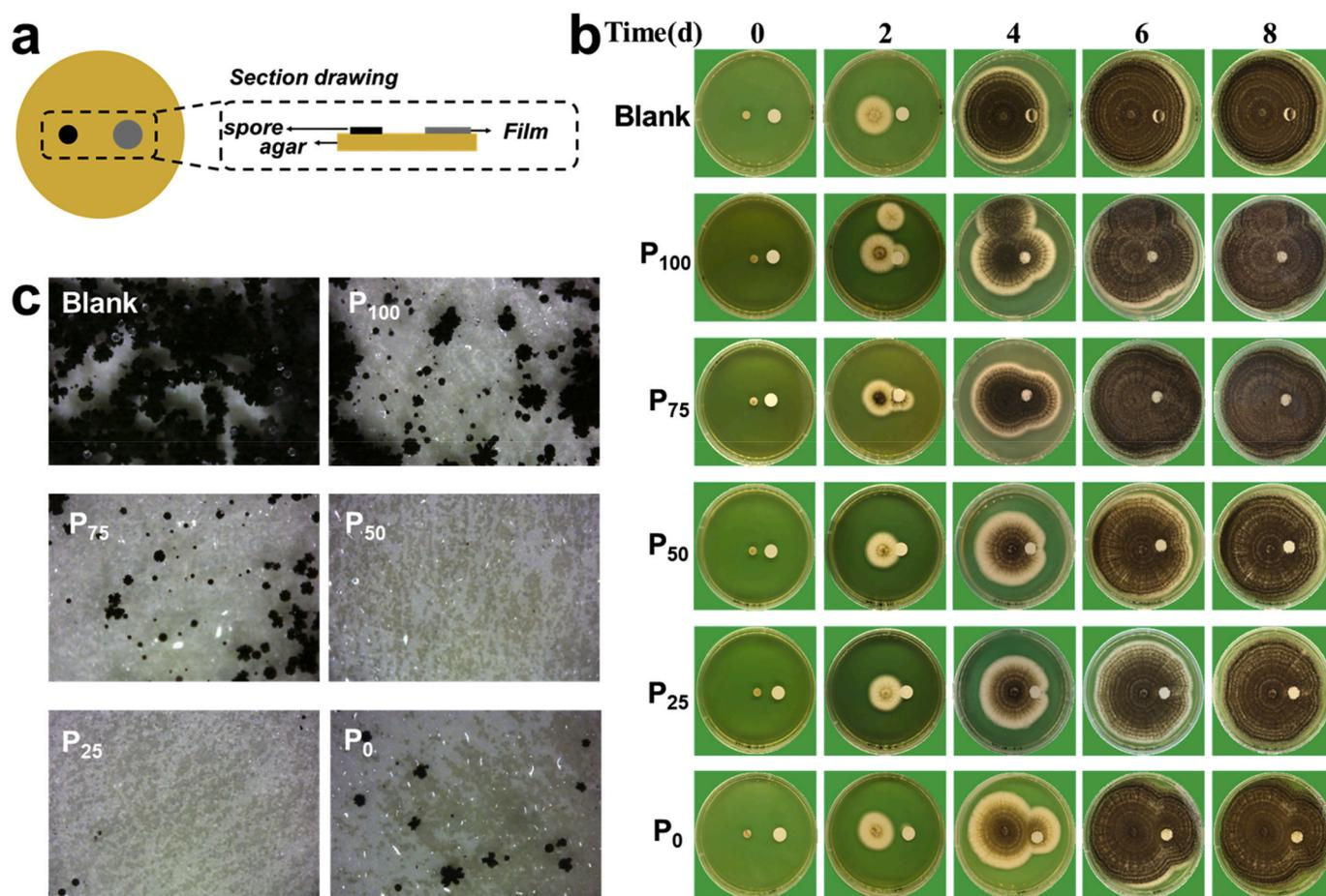
Fig. 3. (a) Schematic illustration of “Landing experiment” experiment for *A. niger* repelling assay of coatings. Contamination of surfaces of different materials (b) and their micrographs (c).
