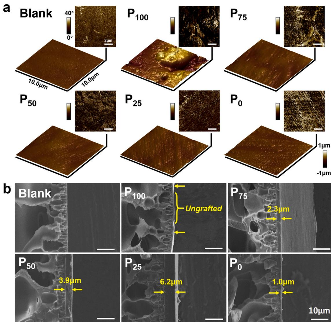
**Fig. 2.** Surface morphology of the coatings. AFM surface height and phase images (a), and SEM cross-section images (b) of blank, P<sub>100</sub>, P<sub>75</sub>, P<sub>50</sub>, P<sub>25</sub> and P<sub>0</sub> samples.
