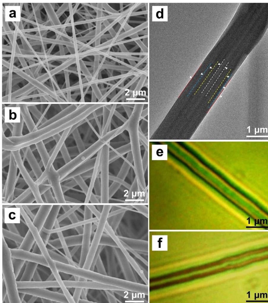
Fig. 2. SEM images of the nanofiber membranes composed of (a) 1-NF, (b) 2-NF, and (c) 4-NF, respectively. (d) TEM image and (e-f) optical micrographs of a quad-axial nanofiber.
