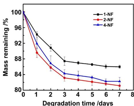
Fig. 3. Mass loss of the different types of nanofiber membranes after *in vitro* degradation for 7 days.
