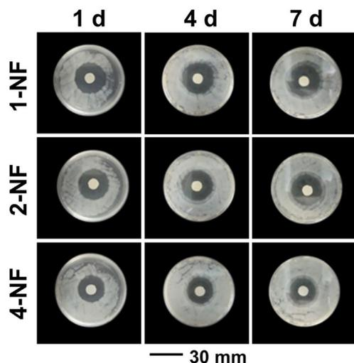
Fig. 7. Optical images of the inhibition zones around the electrospun nanofiber membranes against *S. aureus* after incubation for 1, 4, and 7 days, respectively.
