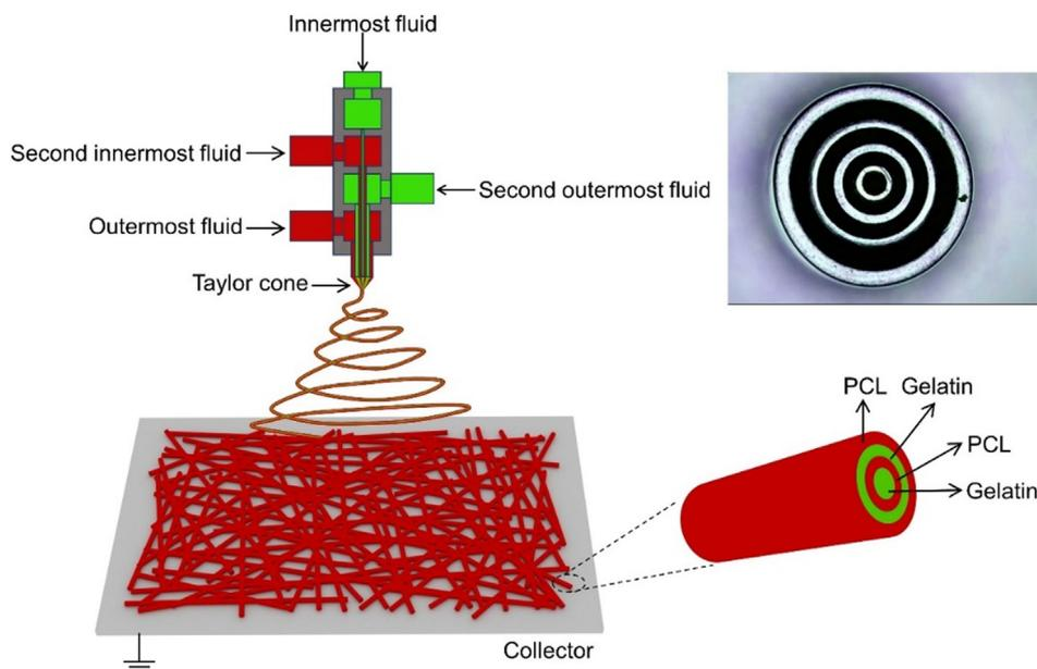
Fig. 1. Schematic diagram of quadriaxial electrospinning. The inset in the upper right shows a photograph of the concentric spinneret.
