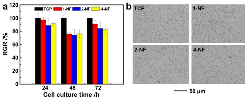
Fig. 5. The *in vitro* cytotoxicity evaluation of the electrospun nanofiber membranes by incubating L929 cells in the extracted solutions of the samples. (a) RGR of L929 cells after incubation for different time, and (b) microscope images of L929 cells after incubation for 72 h.
