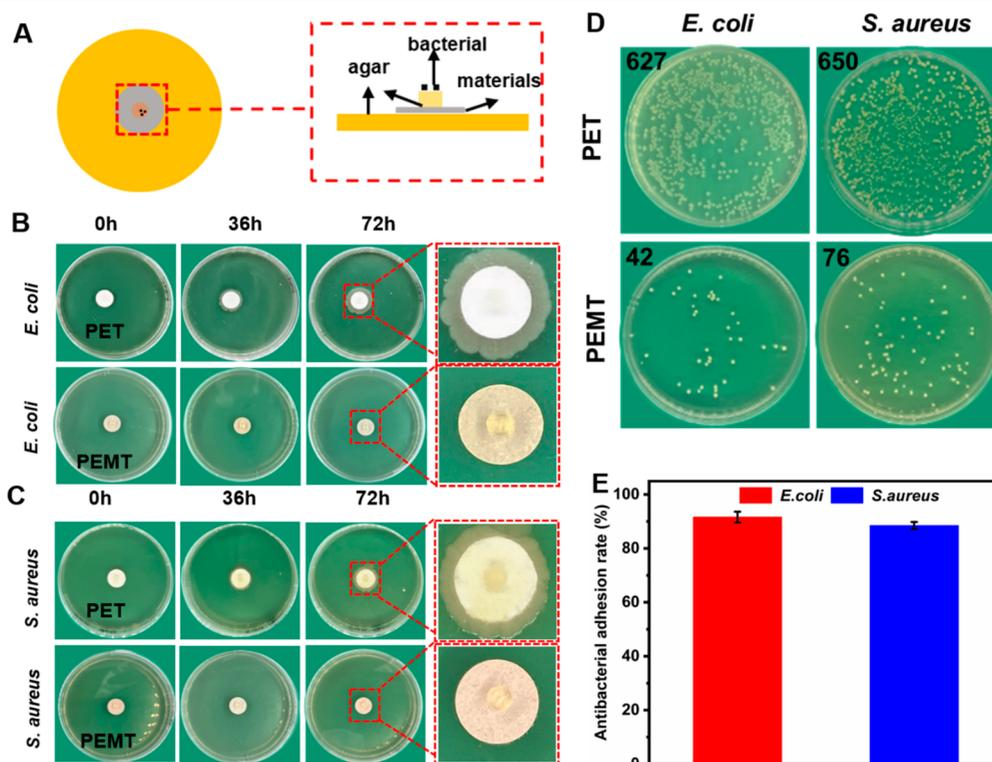
Figure 2. (A) Schematic diagram of antibacterial spreading test. (B) Photographs of agar plates of *E. coli* in the PET and PEMT groups within 72 h. (C) Photographs of agar plates of *S. aureus* in the PET and PEMT groups within 72 h. (D) Result of plate count of PET and PEMT against *E. coli* and *S. aureus*. (E) Antibacterial adhesion rate of PET and PEMT against *E. coli* and *S. aureus*.
