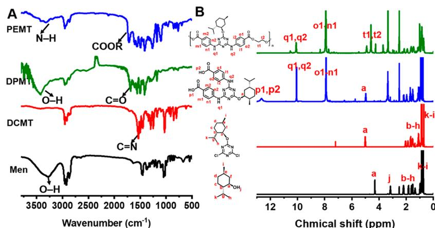
Figure 1. (A) FTIR spectra of Men, DCMT, DPMT, and PEMT. (B) <sup>1</sup>H NMR spectra of Men, DCMT, DPMT, and PEMT.
