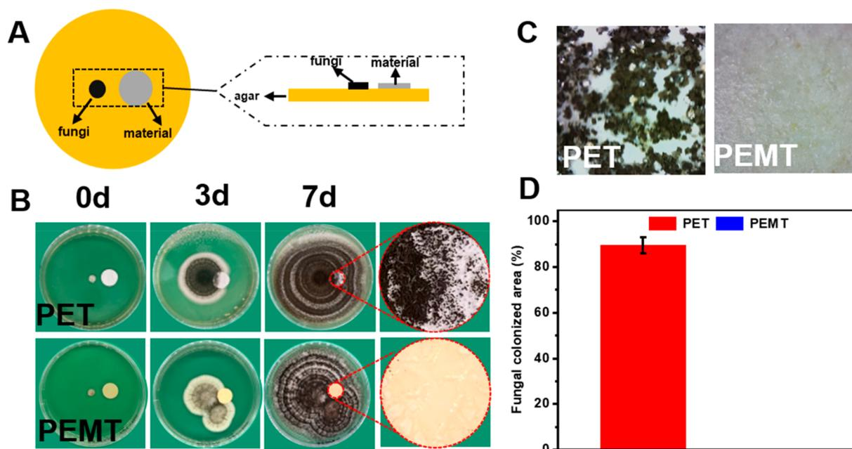
**Figure 3.** (A) Schematic illustration of “antifungal landing test”. (B) Photographs of the growth of *A. niger* in the PET and PEMT groups within 72 h. (C) Micrographs of PET and PEMT surfaces at day 7. (D) Quantification of fungal colonization areas on PET and PEMT surfaces.
