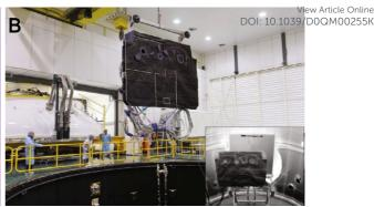
**Figure 18.** Biosafety materials for aerospace safety. (A) SolarBlack material samples during testing in the Synergist Temperature Accelerated Testing (STAR) facility in the ESA/ ESTEC center. (B) Solar orbiter heatshield based on SolarBlack technology.
