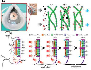
Figure 10. Biosafety materials for PPE with antimicrobial capacity. (A) Schematic illustration of metal-organic framework (MOF)-based filter. (B) Schematic illustration of the filtration mechanism of the polymeric material mask.
