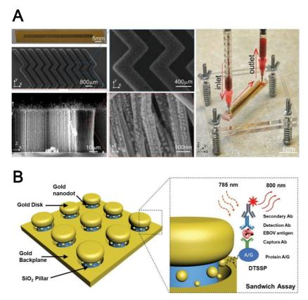
**Figure 5.** Biosafety materials for virus capture and detection. (A) High-throughput microfluidic VIRRION platform containing carbon nanotube arrays for influenza virus capture and identification. (B) Schematic illustration of 3D plasmonic nanoantenna array for EBOV sensor. Adapted from ref. Chou *et al*.
