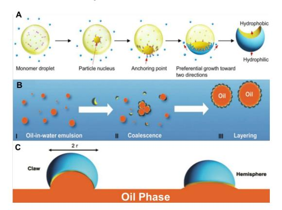
**Figure 13.** Biosafety materials for separating spilled oil from water. (A) Schematic illustration of the principle of hydrophilic/oleophilic magnetic Janus particles. (B) Schematic of the separation of tiny oil droplets by Janus particles. (C) Schematic of the two different types of Janus particle.
