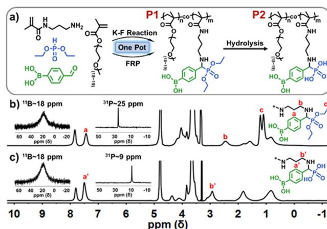
**Fig. 1.** a) Preparation of P1 ([APMA]/[PEGMA]/[4-FPBA]/[DEPP]/[ABVN] = 100/50/110/140/1.5, 60 °C, 12 h) and P2 ([ $\alpha$ -aminophosphonate]/[TMS-Br] = 1:10, 65 °C, 12 h); b)  $^1\text{H}$ ,  $^{11}\text{B}$  and  $^{31}\text{P}$  NMR spectra ( $\text{D}_2\text{O}$ , 400 MHz) of purified P1; c)  $^1\text{H}$ ,  $^{11}\text{B}$  and  $^{31}\text{P}$  NMR spectra ( $\text{D}_2\text{O}$ , 400 MHz) of purified P2.
