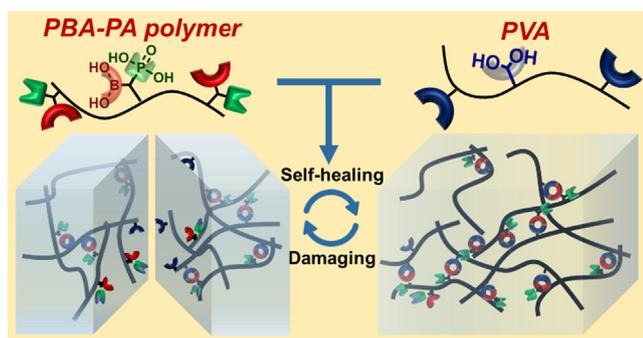
**Scheme 1.** Schematic illustration of the principle of a polyanionic self-healing hydrogel.
