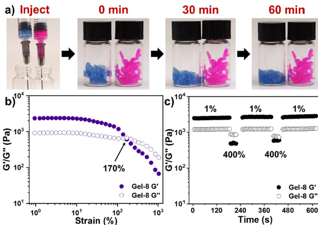
Fig. 3. a) Self-healing process of Gel-8 (blue) after injection with a 22-gauge needle. A hydrogel made from gelatin (8%, red) was used as the control; b) evolution of the  $G'$  and  $G''$  moduli of Gel-8 with different strains; c)  $G'$  and  $G''$  moduli of Gel-8 with alternate strains of 1% and 400%. (For interpretation of the references to colour in this figure legend, the reader is referred to the web version of this article.)
