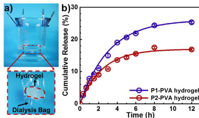
Fig. 5. a) Experimental setup used to study the release of CDDP release; b) cumulative release profiles of CDDP from the P1-PVA hydrogel (blue) and the P2-PVA hydrogel (red). The data are represented as mean  $\pm$  SD,  $n = 4$ . (For interpretation of the references to colour in this figure legend, the reader is referred to the web version of this article.)
