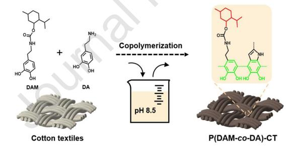
Scheme 1. Schematic illustration of the one-step finishing of P(DAM-co-DA)-CT.
