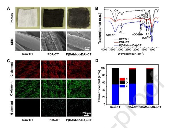
**Fig. 1.** Characterization of P(DAM-*co*-DA)-CT and the control groups of raw CT and PDA-CT. (A) Digital photos and SEM images. (B) ATR-FTIR spectra. (C) EDS
