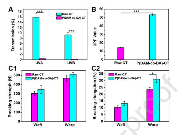
**Fig. 6.** UV-resistant and mechanical properties of P(DAM-*co*-DA)-CT. (A) T(UVA), T(UVB) and (B) UPF value of raw CT and P(DAM-*co*-DA)-CT. Error bars indicate standard deviations (n = 4, \*\*\* p < 0.001). (C1) Breaking strength and (C2) breaking elongation of raw CT and P(DAM-*co*-DA)-CT. Error bars indicate standard deviations (n = 5, \* p < 0.05).
