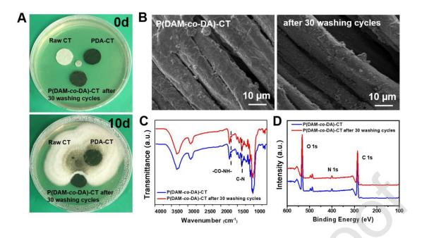
**Fig. 5.** Washing durability test of P(DAM-*co*-DA)-CT according to the FZ/T 73023-2006 standard. (A) Fungal anti-adhesion properties against *A. niger* of P(DAM-*co*-DA)-CT after 30 washing cycles. (B) SEM images, (C) ATR-FTIR, and (D) XPS survey spectra of P(DAM-*co*-DA)-CT before and after 30 successive washing cycles.
