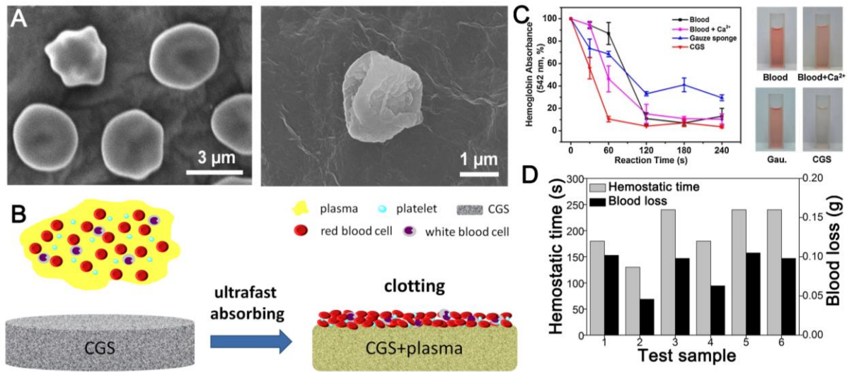
Fig.3 (A) SEM images of blood cells and platelets adhered on CGS. (B) Hemostatic mechanism of CGS. (C) In vitro dynamic whole-blood clotting evaluation and (D) in vivo hemostatic performance of CGS [8]
